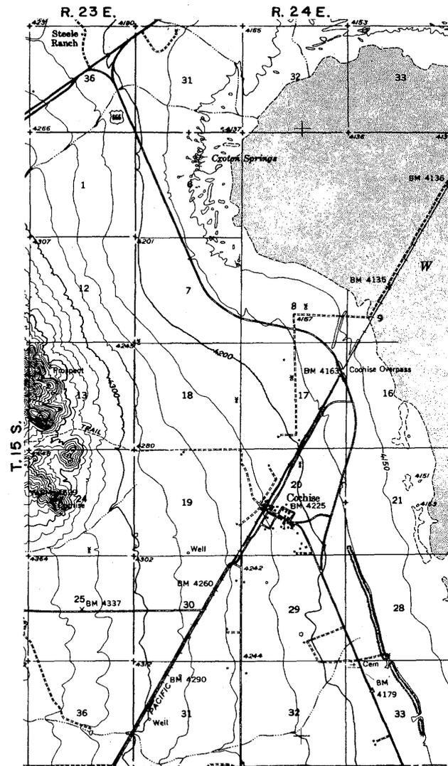
Fig. 15. Index map of west side of playa; beach ridge follows 4,175-ft contour and is shown in secs. 28 and 33, T. 15 S., R. 24 E.
